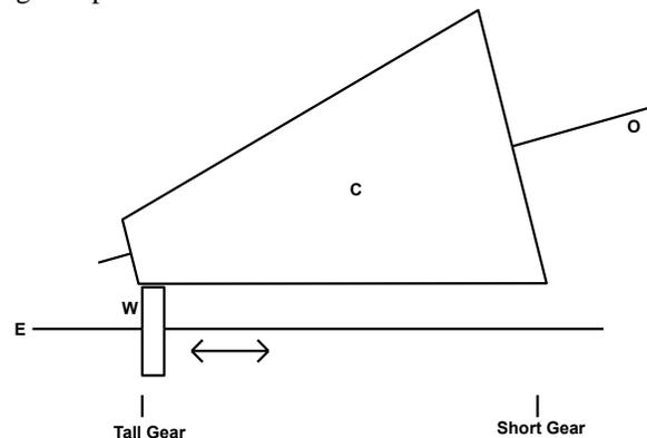
Fig. 3. A traction based CVT in tall gear
