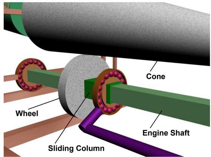
**Fig. 5. Three dimensional view of wheel cone mechanism**
