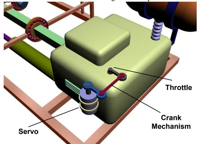
**Fig. 6. Servo throttle control utilizing crank mechanism**
