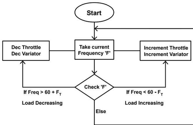
**Fig. 9. CVT based genset running mode algorithm**
