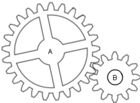
Fig. 2. Two gears having gear ratio 0.48:1
